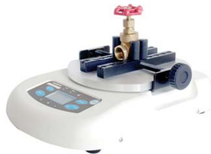
Valve Open/Close testing
